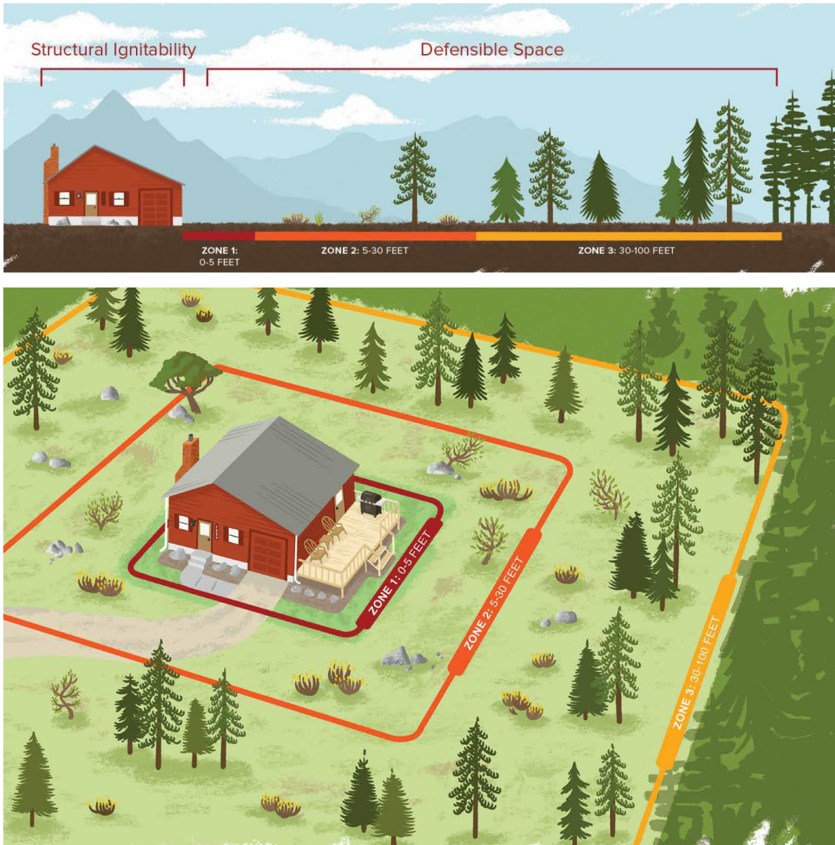
Figure 3.a.2. Home ignition zones recommended by the Colorado State Forest Service. Using ignition-resistant building materials and removing burnable fuel around primary structures, outbuilding such as sheds, and campers / RVs is crucial for increasing your home's chance of surviving a wildfire and creating safe conditions for wildland firefighters. Source: Colorado State Forest Service, The Home Ignition Zone .
